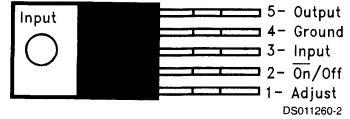
Front View Order Number LM2991T Flow LB03 See NS Package Number T05D
